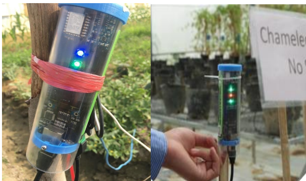
Figure 14: A Chameleon soil moisture sensor installed in a field trial at Long Phu, Soc Trang province (left) and in a greenhouse trial at Can Tho University (right).
